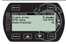
You can set the engine stroke between 1 and 8. RPM delta is the number of engine revolutions you want to have in the intervals if you use the shift light function. In this screen you can also set the number of magnets on the speed sensor disc to a different number than 6, which is the standard number of magnets on the Unipro sensor disc. Use and and buttons to find the setting you want to change. Use
