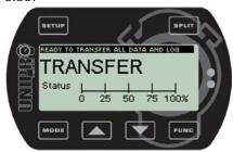
If the Laptimer is set to use USB, you will see this screen when the USB cable is connected. This shows the status of the USB link (PC icon on when USB cable is in) and after this you will choose Receive from the PC Analyser program to start the transmission. When the display shows "Finished" the transmission is finished.
