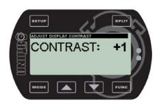
Here you can adjust the screen contrast from +5 to -5. Adjust the contrast with and .
