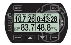
When the finish line is passed for the first time, the display shows 0:00:00 to indicate that the timer is started.
