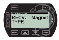
The Unipro Laptimer can use all types of receivers. You can choose between IR (infrared), Loop (AMB active loop) and magnet (magnet stripe in the track).
