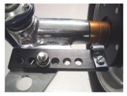
The sensor fitting is mounted in a suitable hole in the stub axle. Depending on the kart model, it can be necessary to drill a hole in the stub axle.
