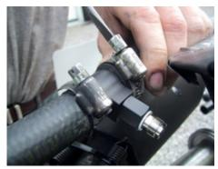
Tighten the two hose clamps to secure the T-junction in the right place.
