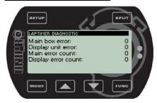
The Laptimer diagnostic screen has mainly information for service purpose. It will show the last error codes for errors from the main box and the display unit, and will show the total number of errors from the main box and the display unit.
