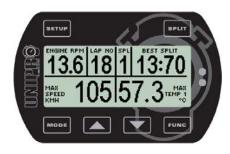
When driving with splits, everything is stored on splits as well as laps. Use the splits button to toggle between all the splits stored in the Laptimer. This example shows the maximum data and the split time for split number 1.
