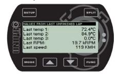
For all three temperature inputs, the temperature is stored at the split second when the engine stops. Therefore, if you have an engine crash you can see the three temperatures at that exact point in time when the engine stop and perhaps it will be clearer why it happened. Also the last RPM and the last speed is stored and shown on this screen.
