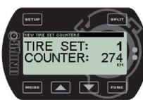
The Laptimer can store the kilometres or miles of up to 8 different sets of tire, each running up to 999 kilometres (or miles).
