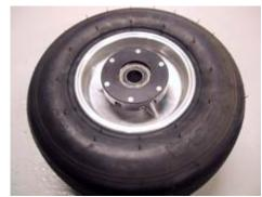
After the sensor disc is mounted, the centering bush is removed again. The wheel is now ready for mounting again.
