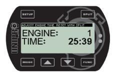
You can use the and buttons to change minutes registered on the chosen engine timer. Each press will count one minute up or down. You can press to reset the timer. Close engine time edit by pressing
