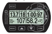
Turning the Laptimer on is done with the During power-on, the display will turn on all segments and the 5 LEDs will blink to show start-up is in progress. During the startup, the batteries are checked and the main box tries to communicate with the display unit. If they cannot find each other, the Laptimer turns off again.
