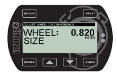
It is entered in millimetres and you need to measure this quite often to keep the system accurate. The best is to use a soft tape measure and do it every time you go out from the pit. It will have influence on the speed, the tire wear counters, and most important the split points.
