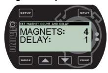
If the receiver type is set to Magnet this is the next step. It is the most important setup before you start driving on a new track. You need to set two values. The number of magnets from the pit to the finish line (1 in this example) and the total number of magnets on the track (4 in this example). See how to set the values in the next to screens.
