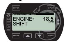
The 5 LEDs at the top of the display can be used as gear shift indicators. In order to do that, you need to set two things. The first is the nominal RPM shift value, that means the RPM value where you want to shift gear. The other is the number of RPMs between the LEDs.
